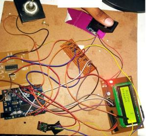
Figure5: LCD display when the finger is placed on the sensor.
