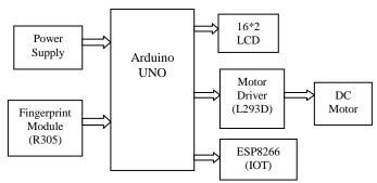
Figure2: Block Diagram of the Project
