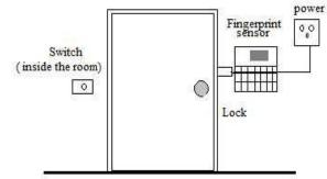
Figure1: Schematic of fingerprint secure system
