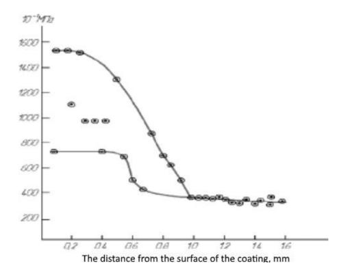
Fig. 2. The change in the microhardness of the carbide coating in depth from the surface of samples made of 35GL steel obtained by casting according to the gasified model.
