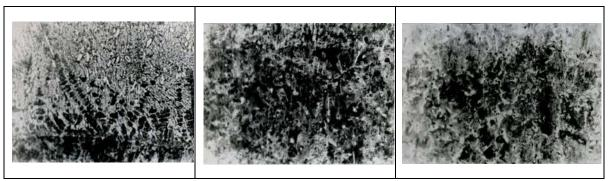
Fig. 1.Microstructures of the carbide coating obtained by casting parts from 35GL steel according to the gasified model.
