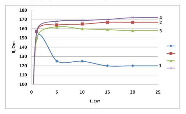
**Figure. 1. Dependence of polymerization resistance on time in 3% NaCl in the presence of a coating:** 1 - uncoated; 2– composition filled with kaolin AKS – 30; 3 - composition filled with AKF – 78 kaolin; 4 – composition filled with AKT – 10 kaolin.
