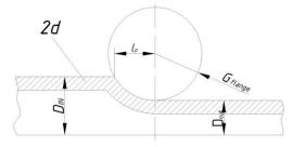
Fig. 5. Caliber seam crimping unit
