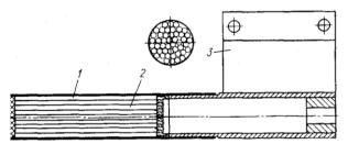
Fig. 3. Ferrite core of cylindrical section: 1 - ferrite rods; 2 - a protective casing; 3 – plates fastenings
