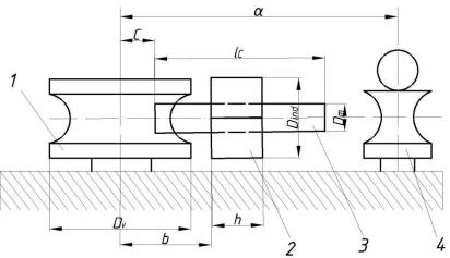
Fig. 1. The scheme of the welding machine of the mill of high-frequency welding of longitudinal pipes: 1 - seam crimping roll with a diameter of  $D_V$ ;
