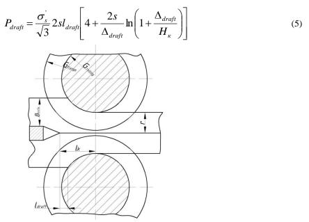
Fig. 4. Diagram of upsetting edges when welding a pipe billet of radius r:
