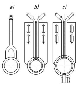
Fig. 2. Designs of inductors for welding longitudinal pipes: a - multi-turn one-piece; b - single-turn one-piece; in - single-turn detachable.
