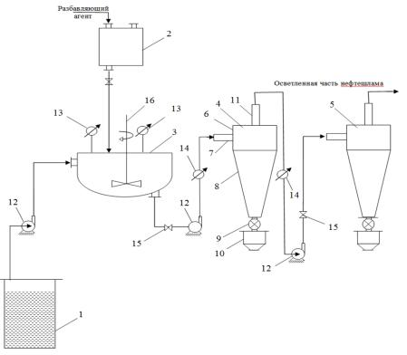
Fig. 1.Purification of oil sludge from mechanical impurities: 1- capacity for oil sludge supply; 2- capacity for supplying a diluting agent; 3.16-capacity with a stirrer; 4,5-hydrocyclones; 6- cylindrical part of the hydrocyclone;
