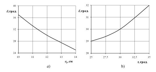
Fig. 2. The dependence of the angle of inclination of the dumped formation to the bottom of the furrow from ay (a) and  $\tau$  (b)
