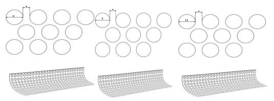
Figure 1. Perforated fibre cleaning screens.
