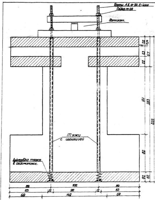
Fig.1 Designs of samples with strands without cores.
