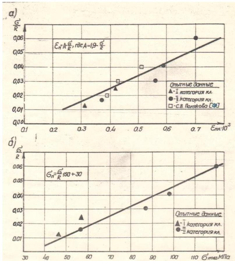
Fig. 3. Change in the masonry creep value (a) and the prestress loss in the reinforcement (b), depending on the compression level.
