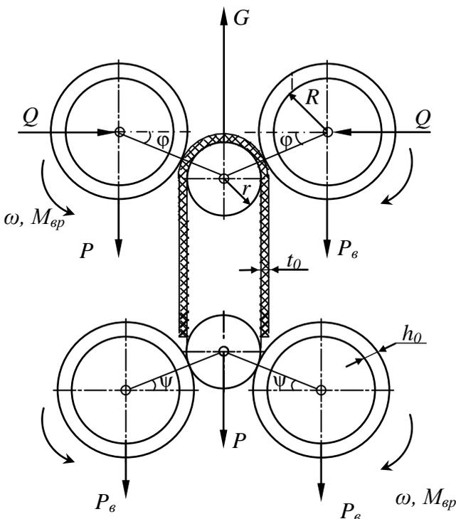
1-picture. Scheme of vertical transmission of fl. the pairs of shaft with an elastic coating
