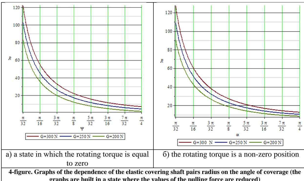
(Figure 5, a,b) the graphs of the binding of the elastic covering radius of shaft pairs to the corner of the coverage shafts are built at different numerical values of the thickness of the monshon. From the results on these charts, we can see that even in these charts, we can see that as the number values of the shafts radius as above decrease, the coverage angle of the shafts will increase as the number values increase. From the graphics we can see that the larger the thickness of the
