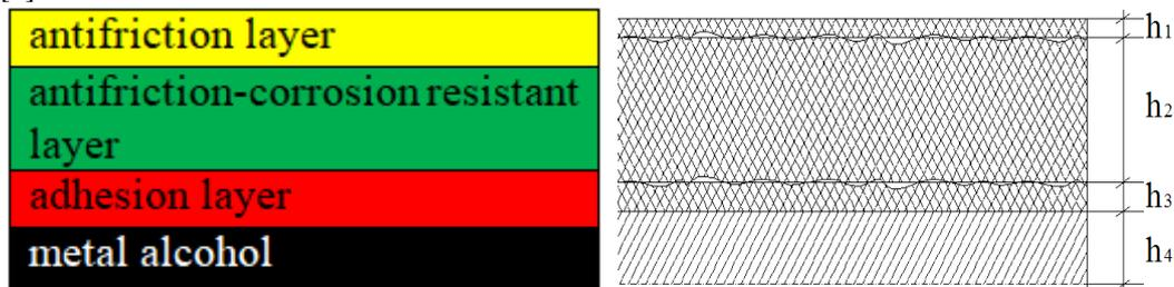
**h1- antifriction layer, h2- antifriction-wear layer, h3- adhesion layer, h4-metal surface**
