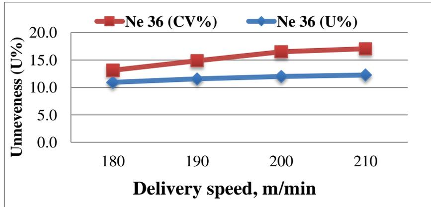
Pic. 1. Effect of the release rate on the uniformity of yarn, U % and CV % by Uster
