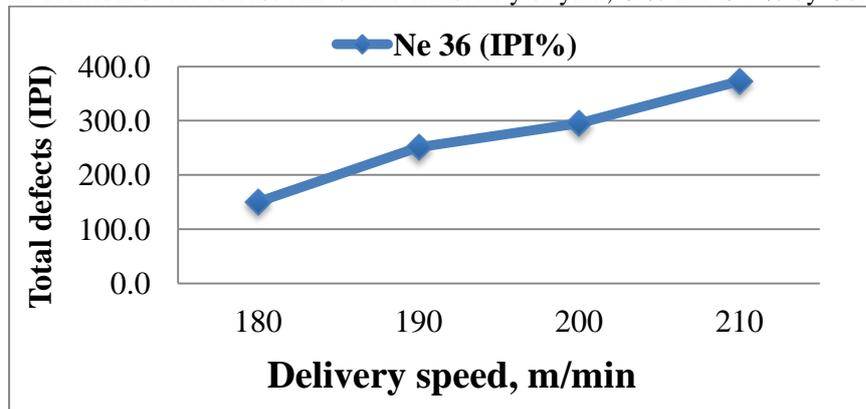
Pic. 2. Effect of delivery rate on defects, yarn IPI
