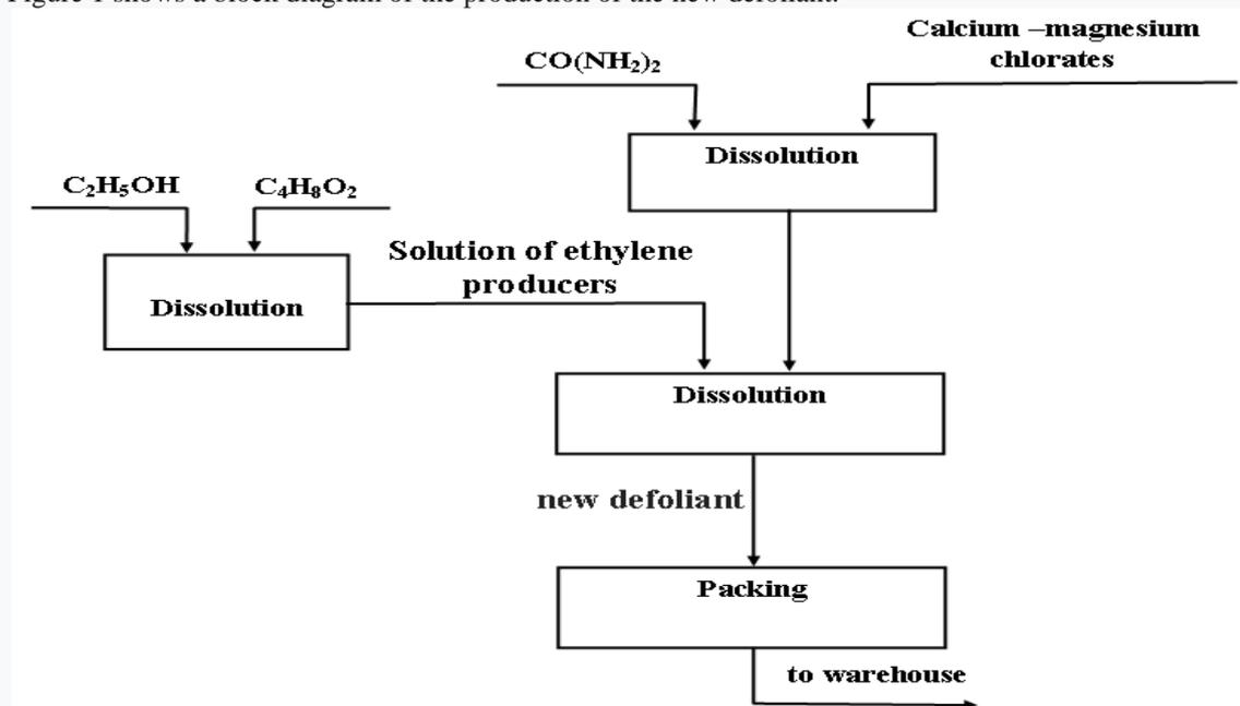
**Figure 1. The block scheme for obtaining 1 t of new defoliant**
