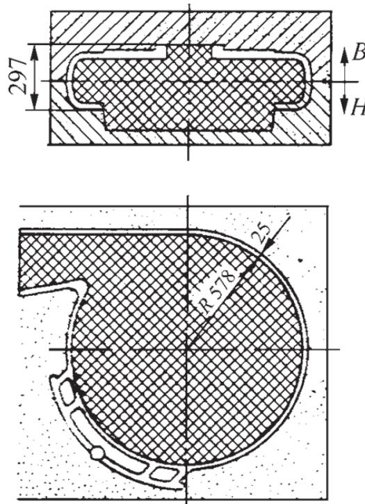
Figure: 2. Diagram of the molding of the pump snail casting 12GR - 8 (weight about 485 kilos)
