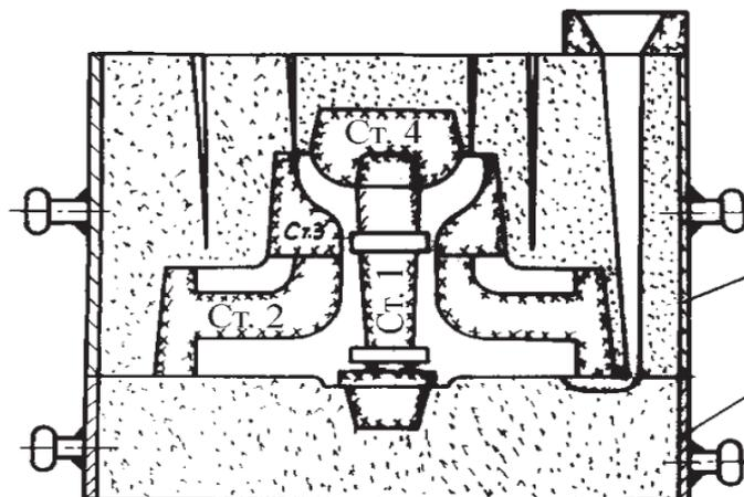
**Figure: 5. Scheme of forming impellers 8NP**
