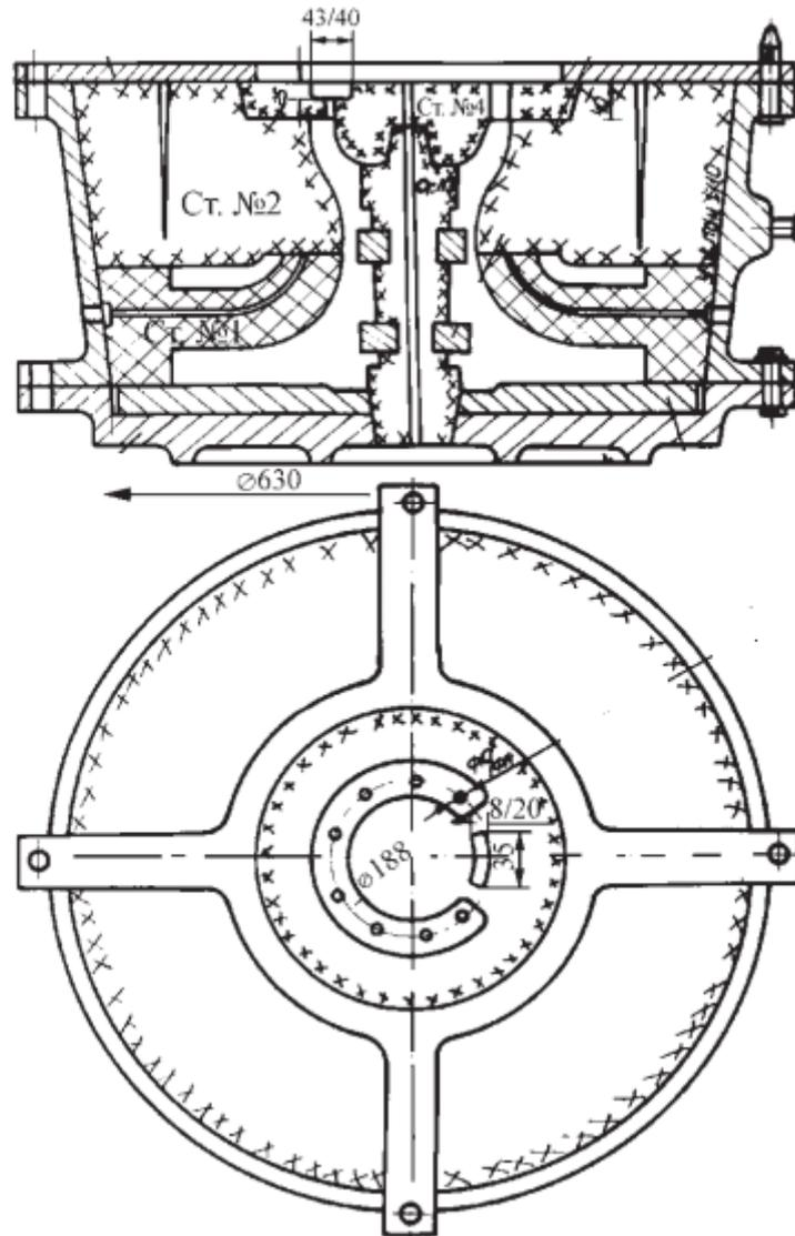
**Figure: 6. Scheme of forming 8NP impellers using a refrigerator (insert)**
