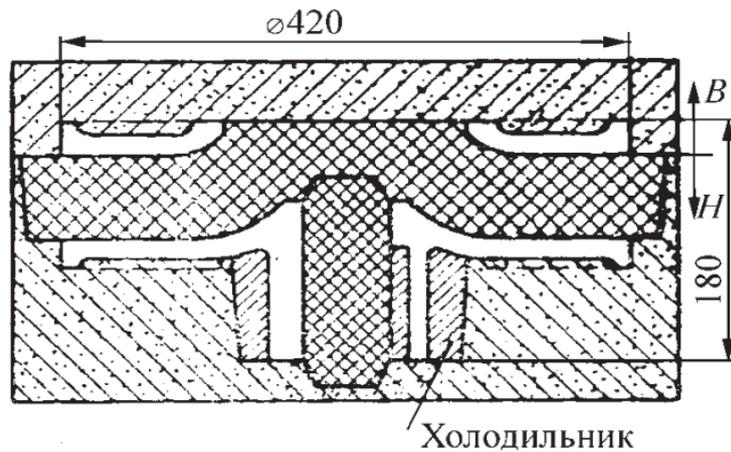
**Figure: 4. Forming scheme with a cooler (at the hub) of the pump impeller 6FSH – 7 a (weight about 90 kilos)**
