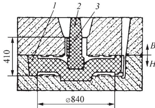
Figure: 3. Diagram of the casting of the impeller (weighing about 280 kilos) of the pump 12GR - 8 (1-3 cm. Text)
