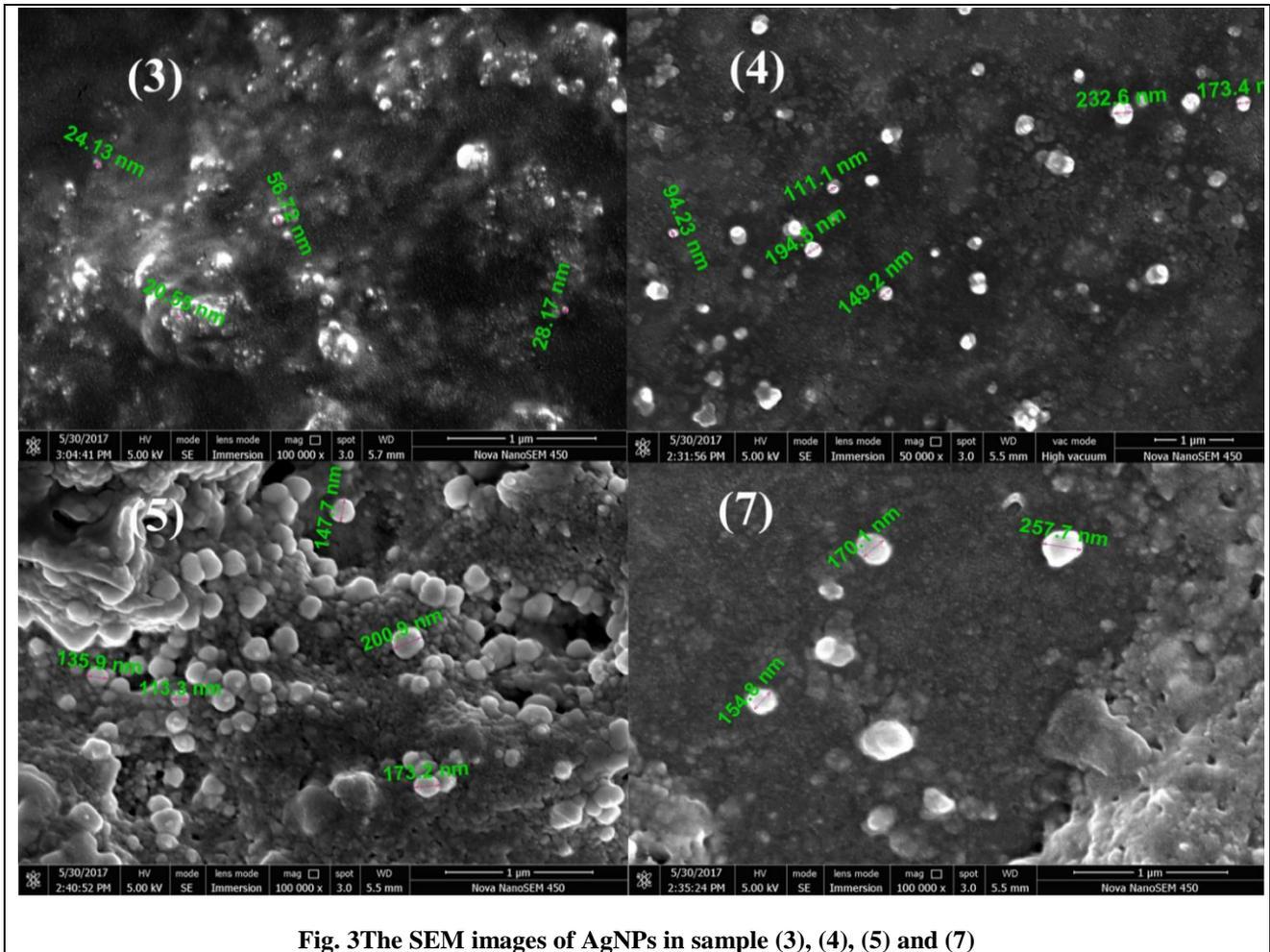
Fig. 3 The SEM images of AgNPs in sample (3), (4), (5) and (7)
