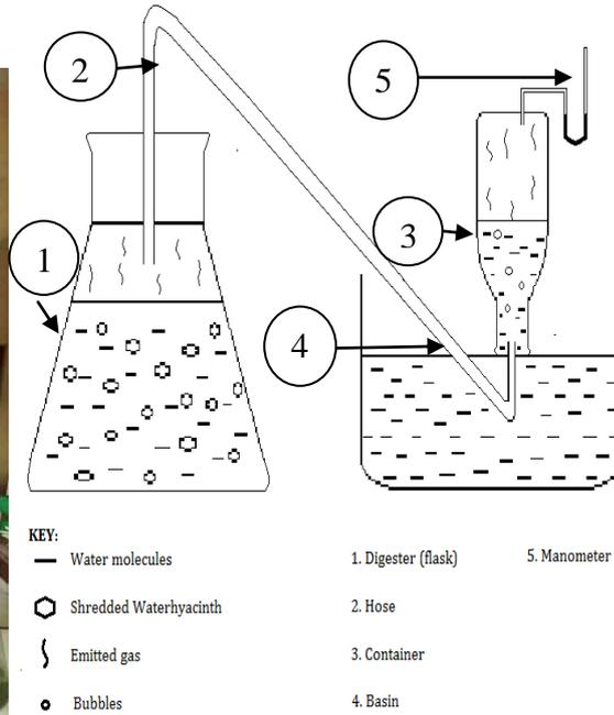
Figure 3: Experimental set up for demonstration of Gas evolution
