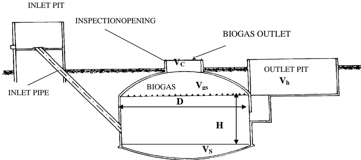
Figure 6: Anaerobic digester
