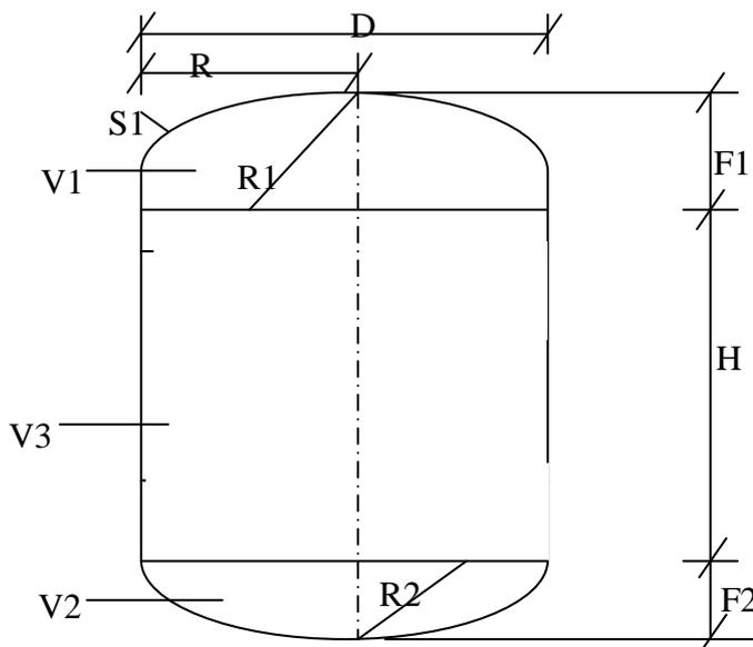
Figure 5: Geometrical dimension of the cylindrical shaped biogas digesters
