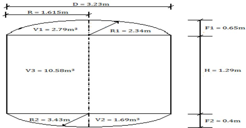
Figure 7: Designed Prototype Digester
