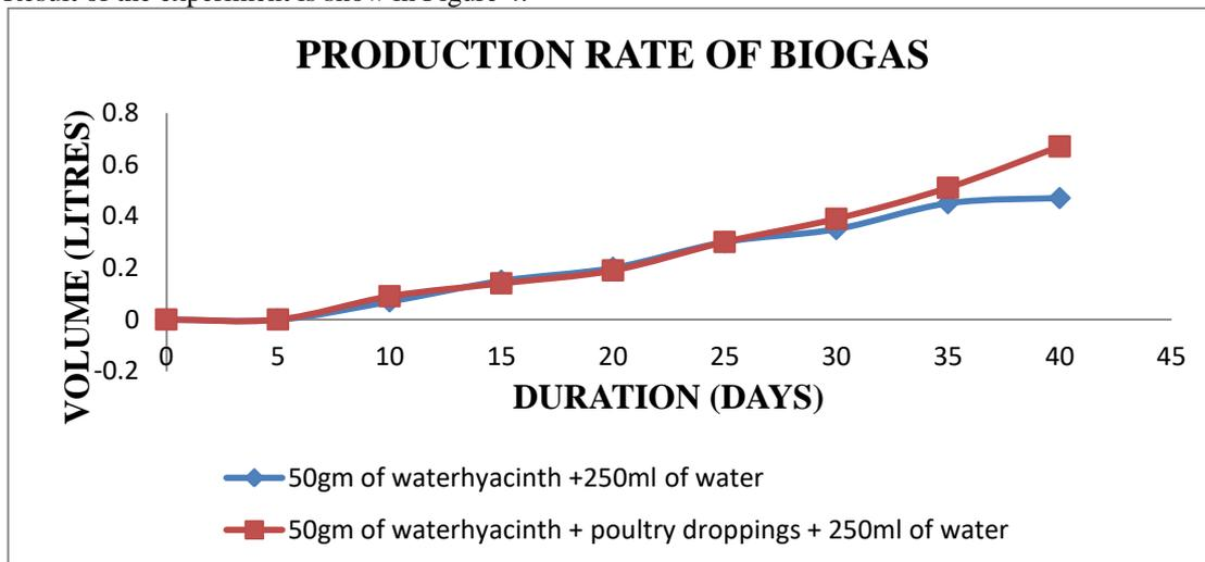
Figure 4. Effect of addition of poultry droppings (inoculums) + 250ml of water
