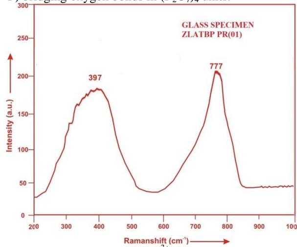
Fig.2: Raman spectrum of  $\text{Pr}^{3+}$  doped ZLATBP (01) glass.
