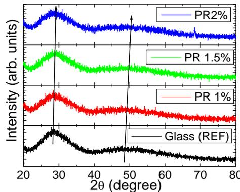
**Fig.1: X-ray diffraction pattern of ZLATBP (PR) glasses.**
