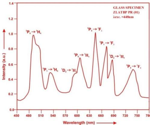
Fig.4: Fluorescence spectrum of ZLATBP PR (01) glass.
