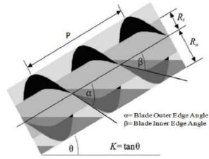
Fig 2.1 Angles in a Screw
