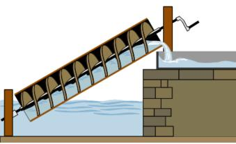
Fig 1.1 Archimedes Screw Pump<sub>[1]</sub>
