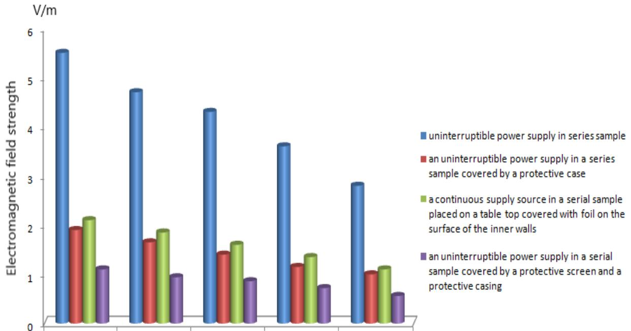
**Figure 4. Values of electromagnetic field strength histogram**
