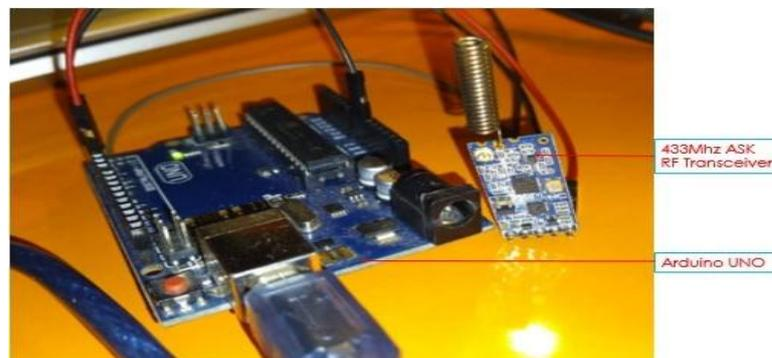
**Fig.3. Setup for transmission of sensor data via 433MHz RF transmitter**
