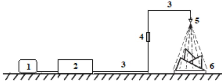
Figure 3. Schematic of the laboratory device: 1 - capacity; 2 - pump; 3 - pipe; 4 - water meter; 5 - sprayer; 6 - Fireplace
