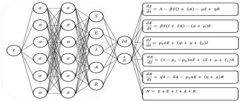
Figure 2: Neural network for system of differential equations
