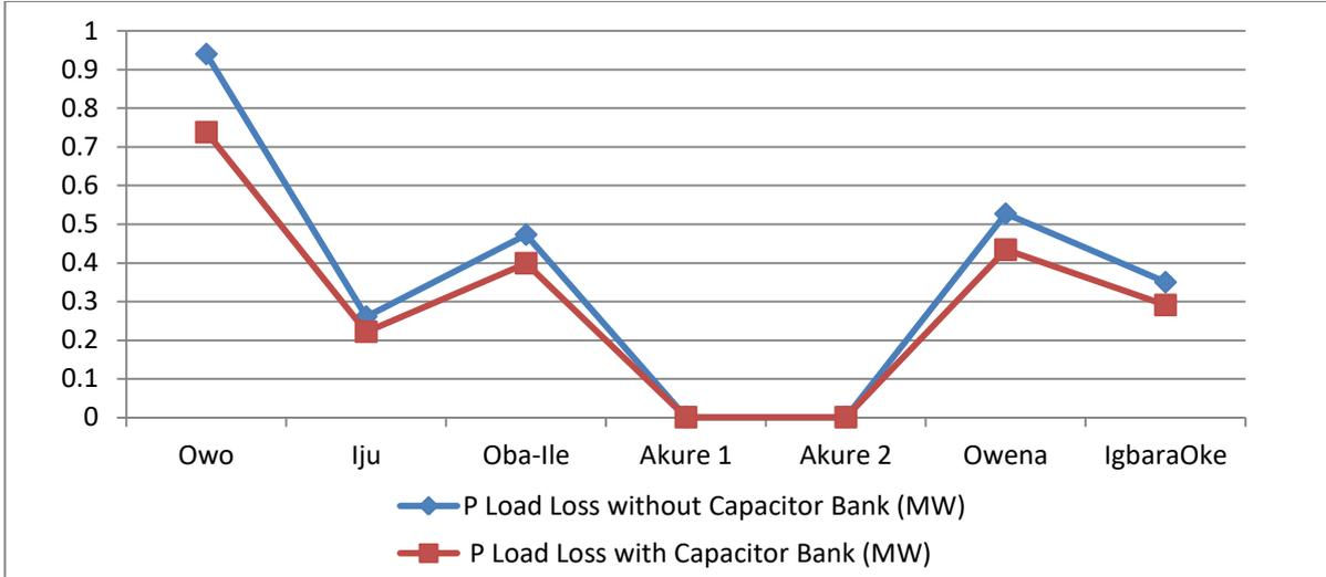
Figure 4. Comparison of Real Power Losses on the Lines
