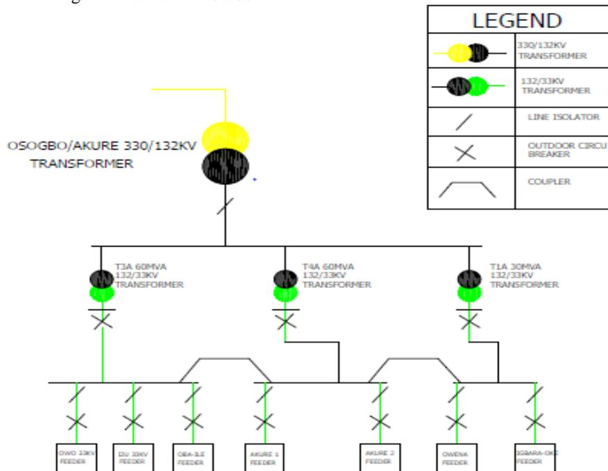
**Figure1. Single line diagram of Akure 132/33KV network**
