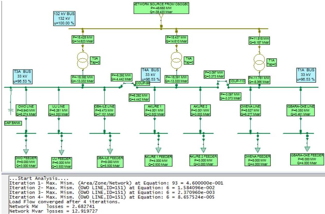
Fig 2: Modelling of Akure 132/33kV network without Capacitor Bank
