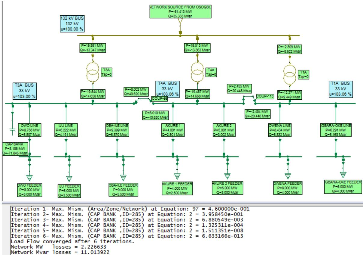
Fig 3: Modelling of Akure 132/33kV network with Capacitor Bank
