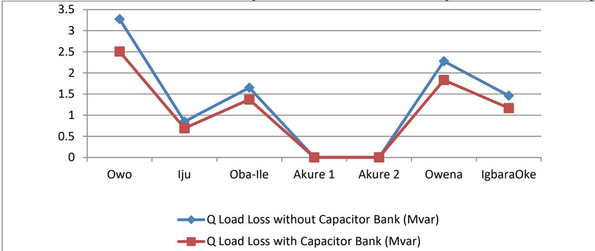
Figure 6 Comparison of Reactive Power Losses on the Lines
