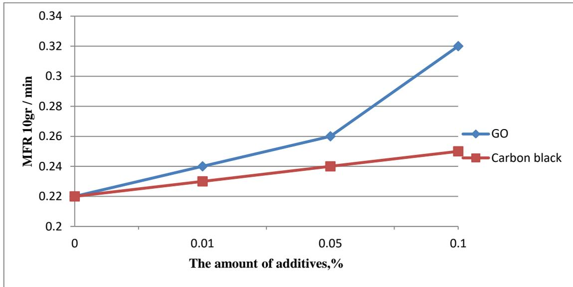
**Fig 1.MFR of HDPE-based compositions with additives of exhaust gases and carbon black.**
