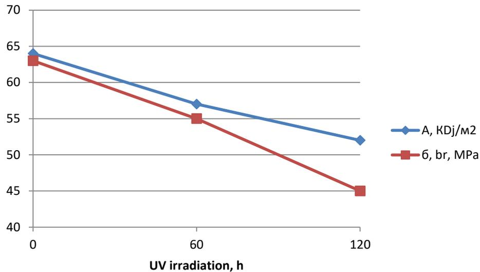
**Fig. 3. Changes in the properties of the HDPE + GO after exposure to UV radiation**
