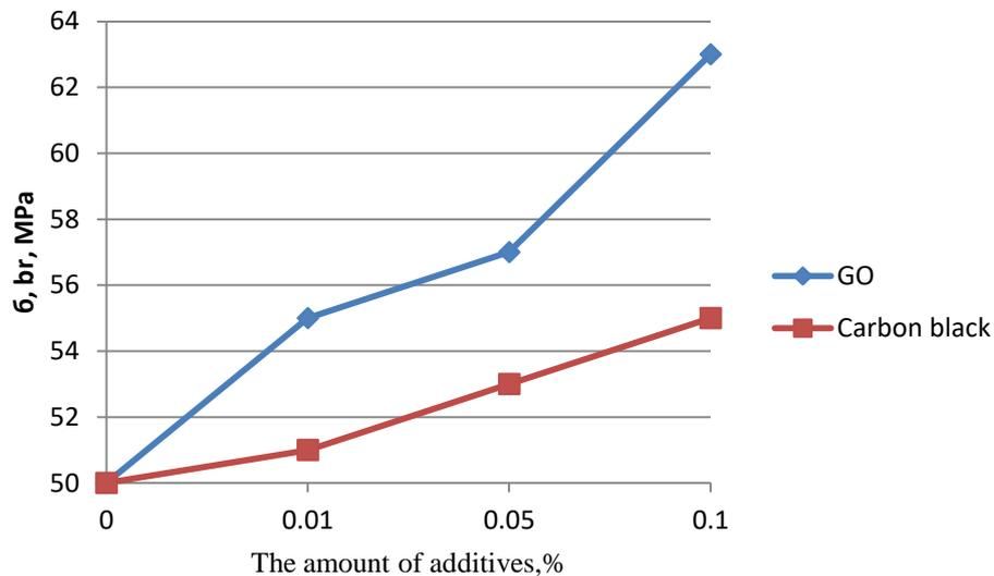
**Fig. 2. Influence of additives on impact strength (a) and tensile strength (b) of composites based on HDPE.**
