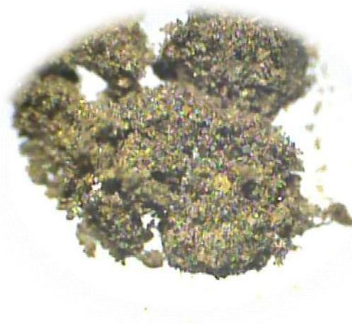
**Fig. 2. Snapshot of a sample of graphite concentrate at 100-fold magnification.**
