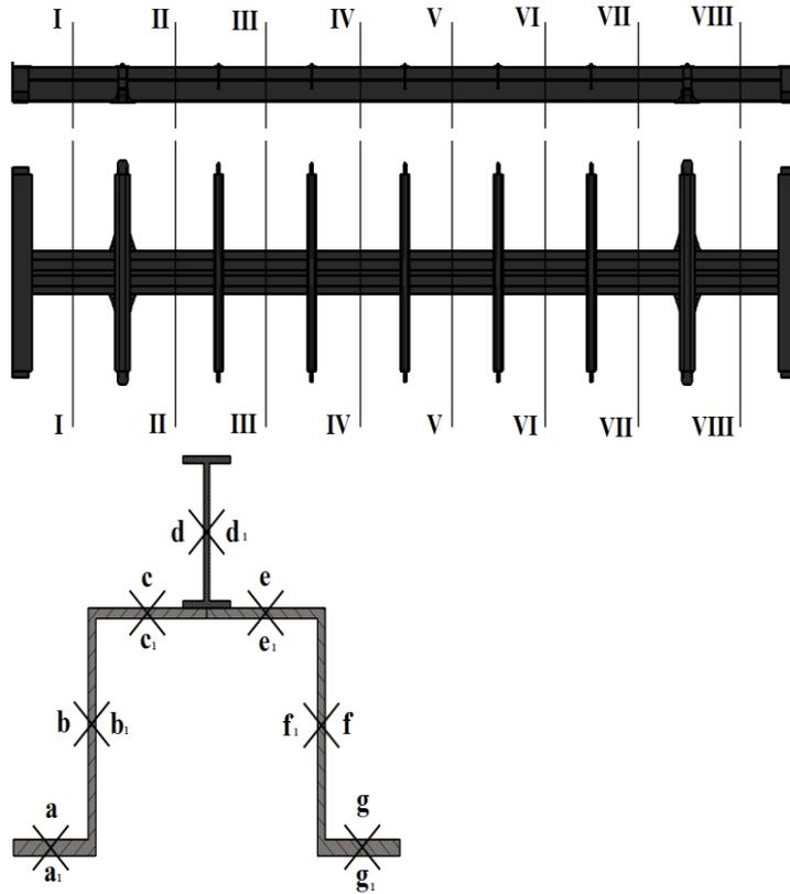
Figure: 3. Scheme for measuring the thickness of wear of sheets on the center beam of the frame of the weighing wagon
