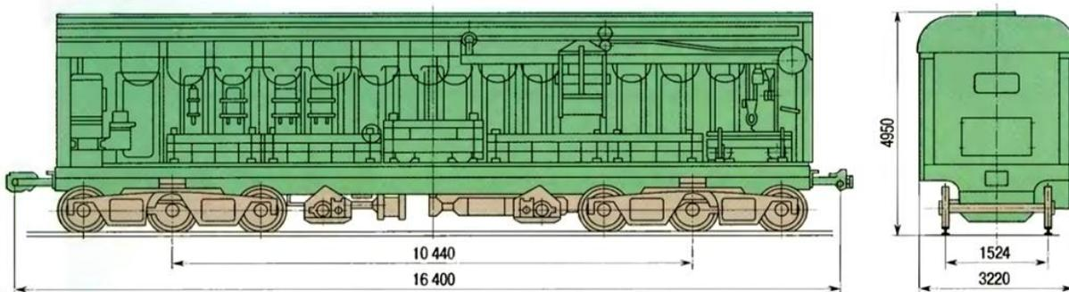
Figure: 1. Weight-checking wagon of 640-VPV type
