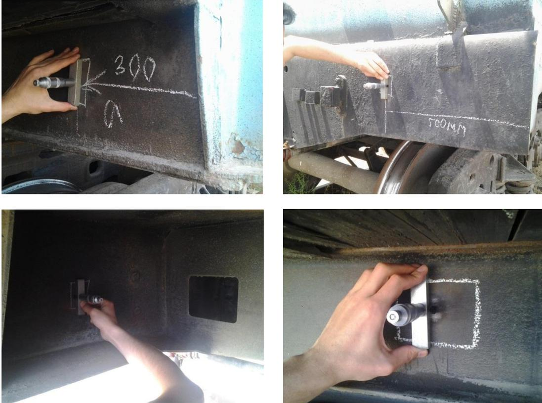
Figure: 7. Measurement of the frame elements of the weighing wagon
