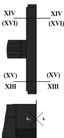
Figure: 5. Scheme for measuring the thickness of sheet wear on the end beam of the weighing wagon frame
