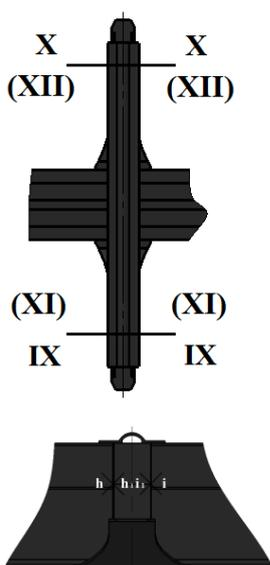
Figure: 4. Scheme for measuring the thickness of sheet wear on the pivot beam of the weighing wagon frame
