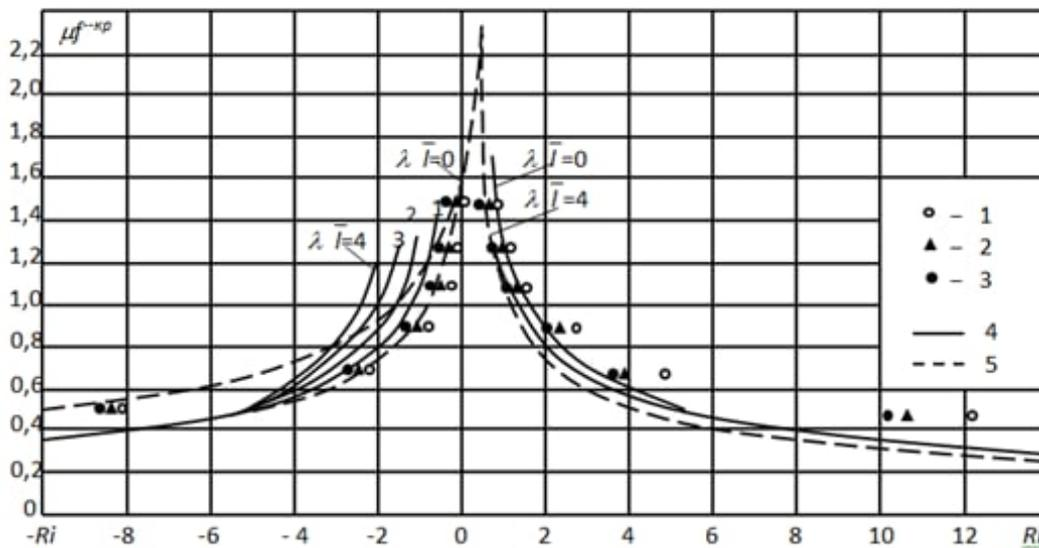
Fig.3. Critical value of nominal slot parameter  $\mu_f^{cr}$  as a function of Richardson number  $Ri$ ; 1,2,3) experiments for  $\bar{\lambda}_l = 0.28, 0.30, 0.36$ ; 4) calculations based on formula (21); 5) computer calculations.
