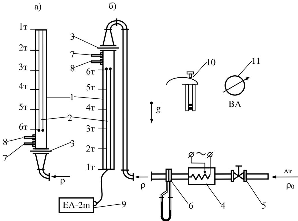
Fig.2. Basic diagram of aerodynamic test stand for investigating distribution under conditions  $Ri < 0$  (a) and  $Ri > 0$  (b): 1) distributor being tested; 2) longitudinal slot equipped with a baffle; 3) rectifying grid; 4) electric heater; 5) shutoff; 6) normal choke diaphragm with manometer; 7,8) dry and wet thermometers; 9) thermalanemometer; 10) psychrometers; 11) barometer.
