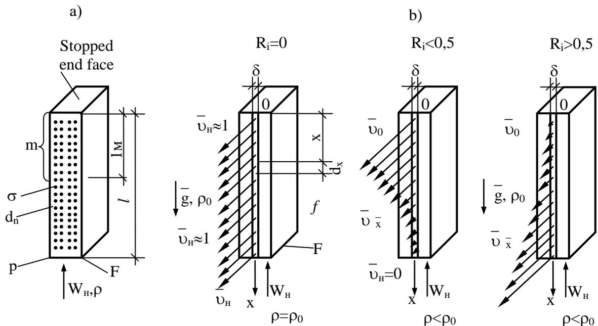
Fig.1. Diagram of water distributor of constant cross section with uniform perforation (a) and with a nominal slot of constant width (b).
