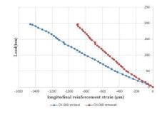
Fig.16: Ultimate load verses Horizontal concrete strain. Fig.17: Ultimate load verses longitudinal reinforcement strain column H1.5,0,1.5.
