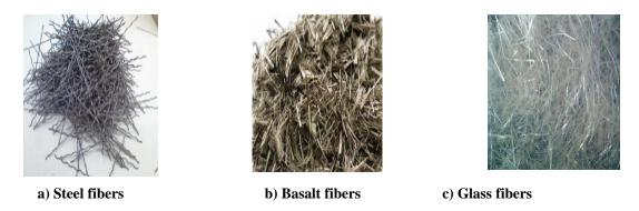
Fig.2: various types of chopped fibers a) steel fibers, b) Basalt fibers and c) Glass fibers.
