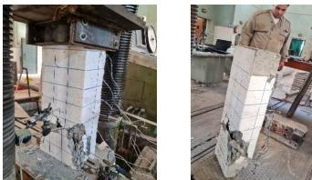
Fig.9: Failure mode for column H0.5, 1.5.
