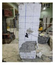
Fig.11: Failure mode for column H1.5,1.5.
