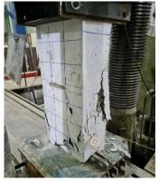
Fig.10: Failure mode for column H1,1.5.
