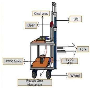
Fig. 3.1. Forklift material handling system
