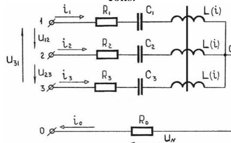
Figure 6. Three-phase ferroresonant circuit with zero-wire c ferromagnetic coupling between the non-linear coils.
