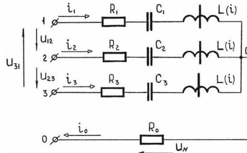
Figure 4. Three-phase ferroresonant circuit with symmetrical power supply.
