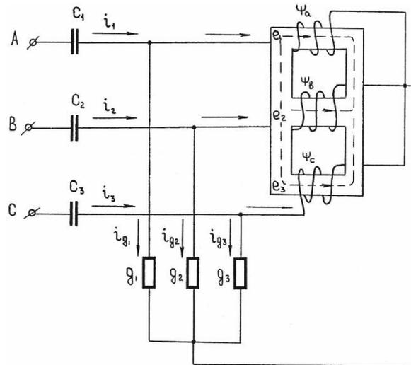
Figure 1. Three-phase ferroresonant AP circuit with magnetic coupling between phases without a neutral conductor.
