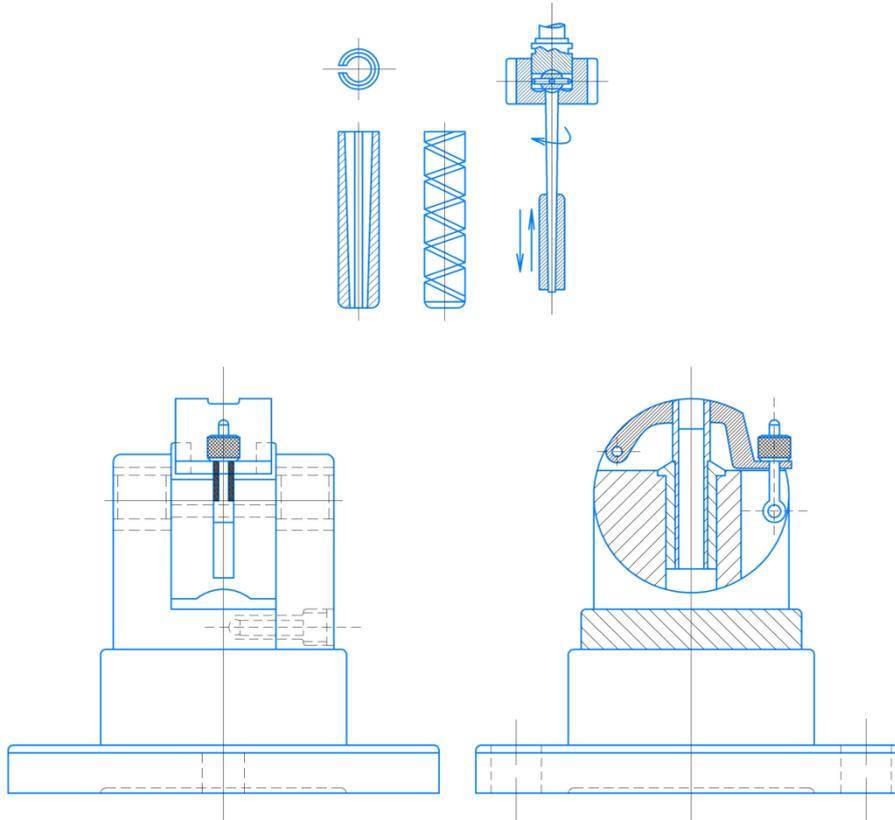
**Fig.1. Bushing Lapping Tool**
