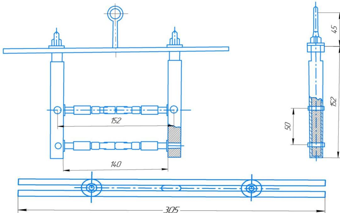
Fig. 3. Typical hanger for plunger chrome plating: 1-insulating material; 2-piece set for chrome plating.
