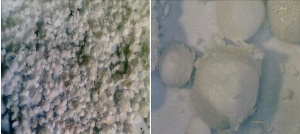
**Figure 1. Milled recycled polystyrene.**
