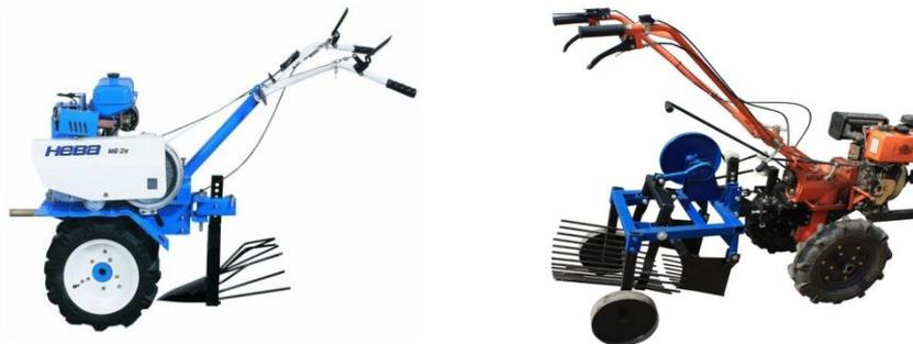
**Figure 1. Motoblocks equipped with excavating working bodies of various constructions**
