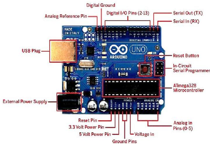
**Fig No. 5 Arduino UnoR3 board [9]**
