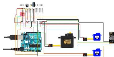
**Fig no. 4 Arm circuit diagram**
