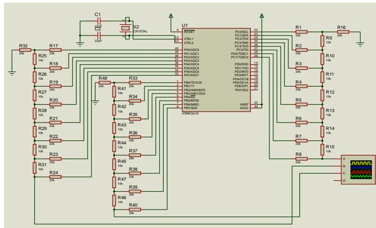
Figure 3. Schematic of 3 Phase Sine Signal Generator
