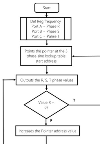
Figure 4. 3-Phase Sine Generator Microcontroller. Program Flowchart
