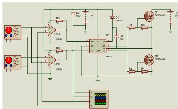
Figure 7. Modulator, Driver and Switching Circuit Schemes
