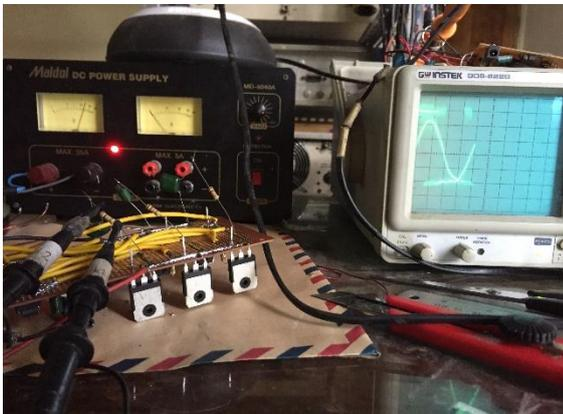
Figure 13. Testing the modulator, driver and switching circuits
