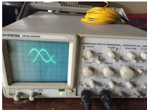
Figure 10. Measurement of Sine Signal Generating Results of 3-Phase Sine Signal Generator
