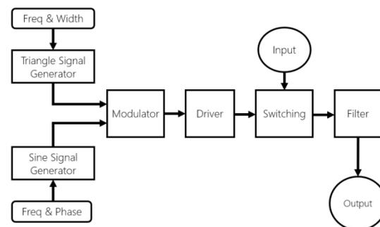
Figure 2. 3-Phase Inverter DC-AC Block Diagram
