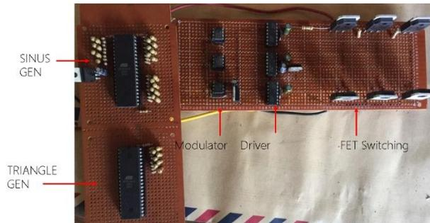
Figure 8. 3-Phase DC-AC Inverter Circuit Figure
