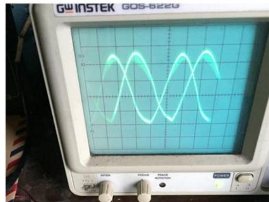
Figure 14. Test Results for 3 Phase DC-AC Inverter Output
