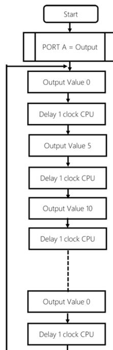
Figure 6. Triangular Signal Generator Program Flowchart
