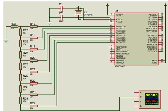
Figure 5. Triangular Signal Generator Design Scheme
