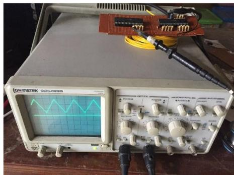
Figure 11. Measurement of Triangular Signal Generating Results of Triangular Signal Generator
