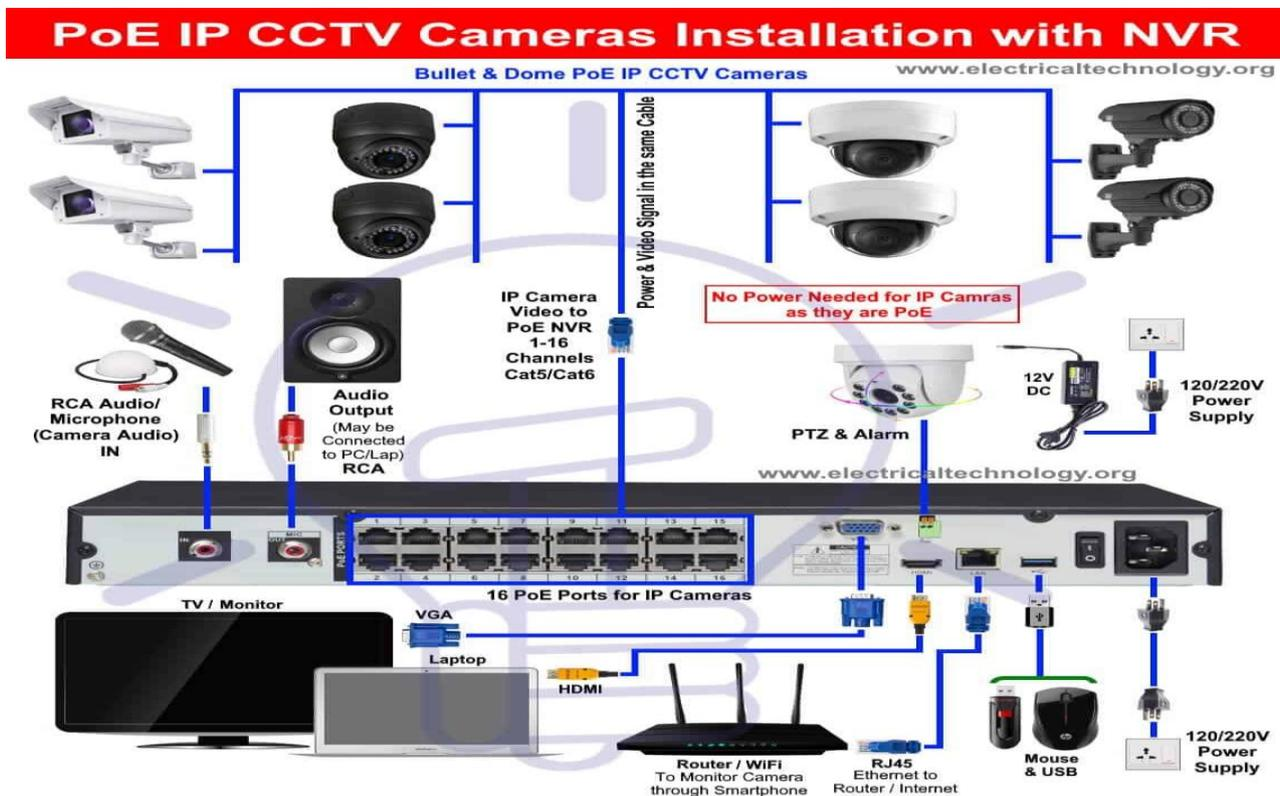
Figure 7: PoE IP CCTV cameras security system with NVR. [20]
