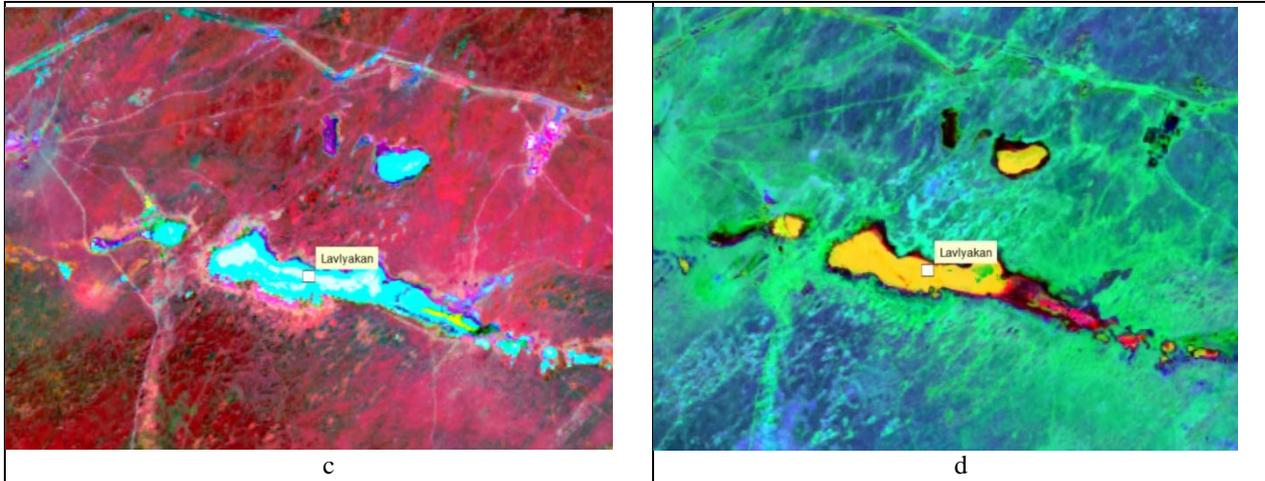
**Fig.4. The results of processing space images (scale 1:50,000) for the site of the Lavlyakan group of lakes: a - composite satellite image Landsat-5 (1994); b – Landsat-8 satellite image (June 20, 2013); c – PCA; d – Hydrothermal Composition.**
