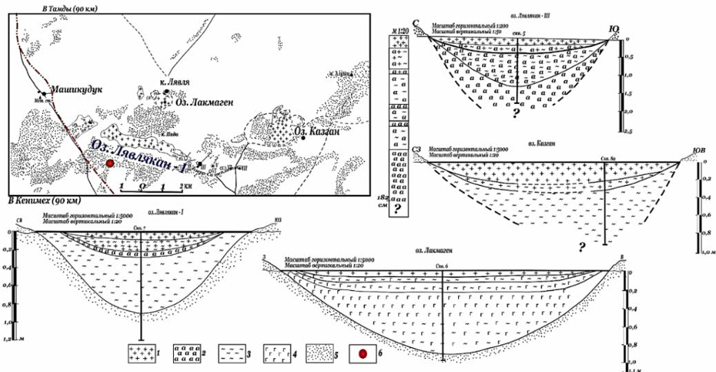
**Fig.3. Scheme of location and structure of the Lavlyakan deposit of astrakhanite and halite:**
