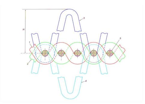
Figure 1, Scheme of formation of terry fabrics, section cut the weft yarn.
