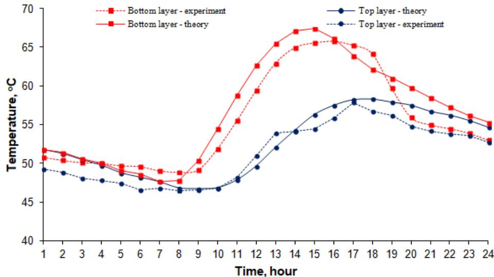
Figure 2. Graph of temperature changes in the upper and lower layers of the heat accumulator capacity of the water tank as a function of time.
