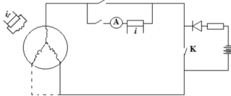
Fig.2. Electric circuit of the experience of attenuation of direct current on a stationary machine.
