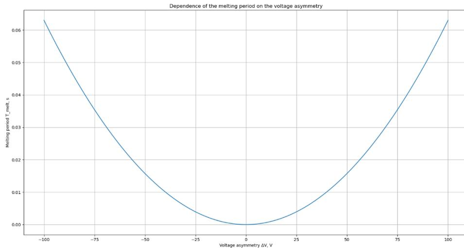
**Figure 1. Graph of the relationship between voltage asymmetry and metal melting time**
