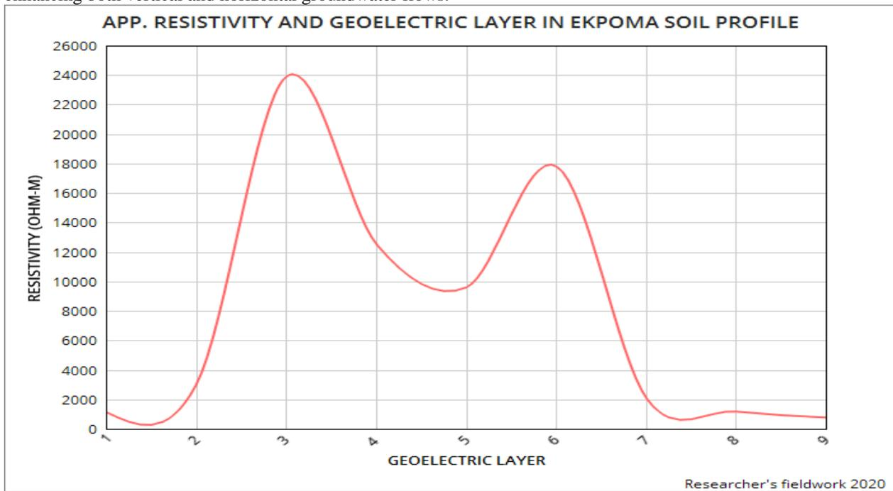
**Fig. 1: Variation of Resistivity with Geoelectric layer for Ekpoma Soil Profile (Culled from Table 1)**
