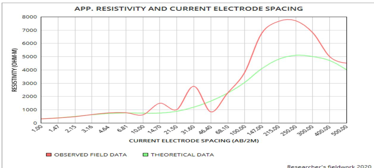
**Fig. 4: Resistivity Variations of apparent resistivity and current electrode spacing in Irrua Soil Profile (Culled from Table 2)**
