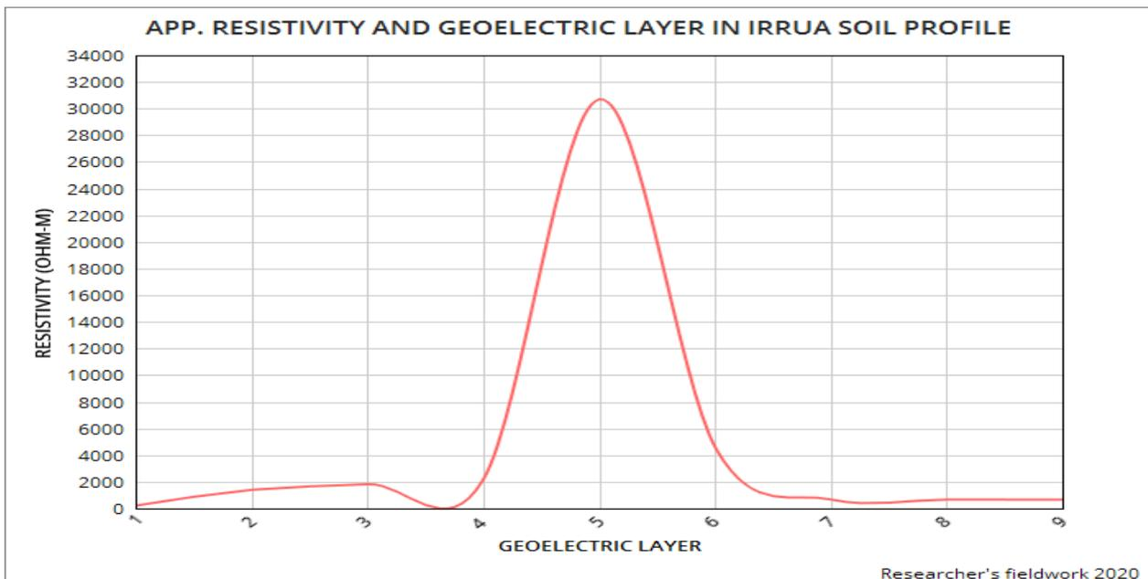
**Fig. 5: Variations of apparent resistivity with geoelectric layer in Irrua Soil Profile (Culled from Table 3)**
