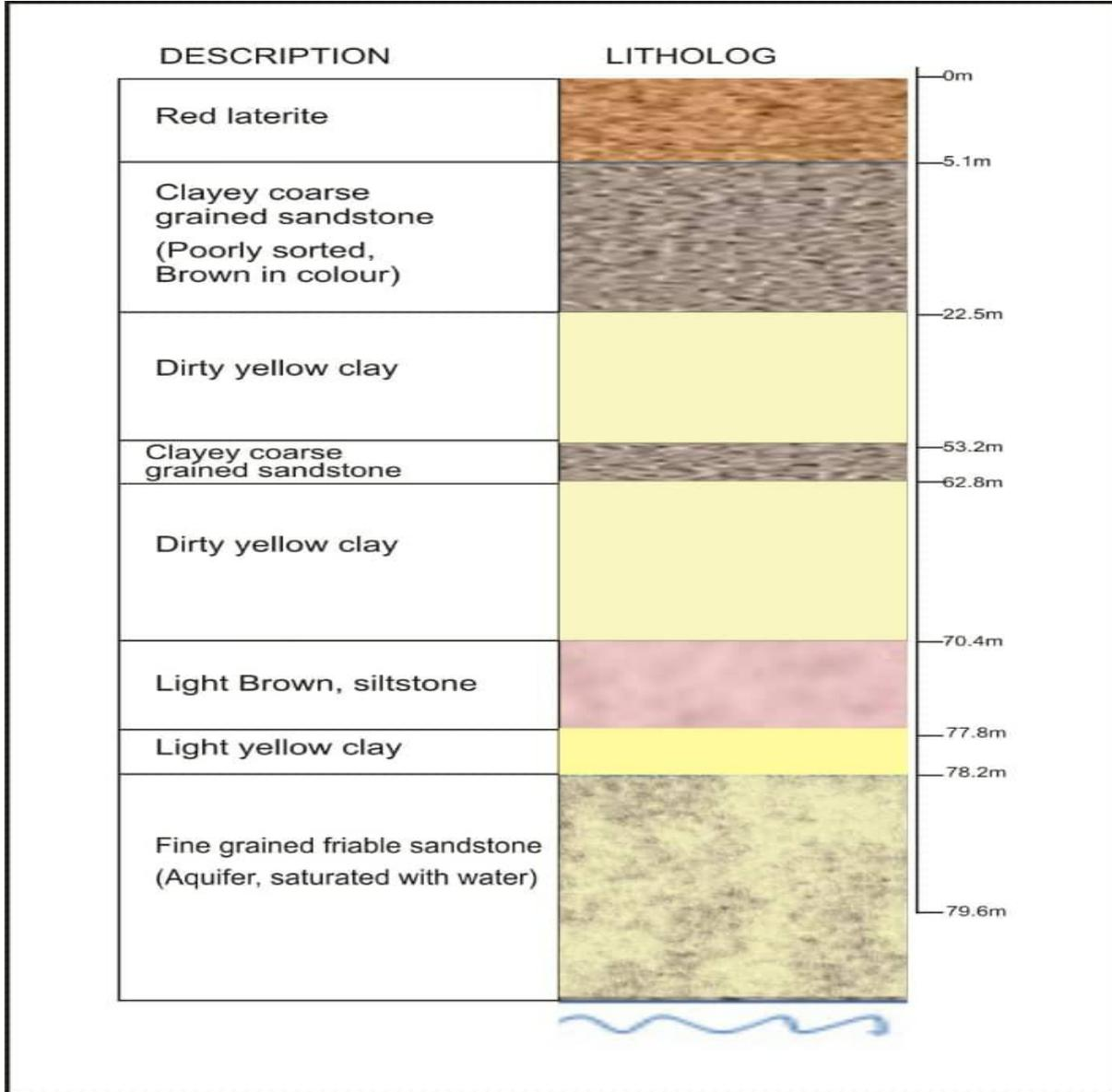
**Fig. 6: Litholog of Groundwater in the study area (Researchers’ fieldwork, 2020)**
