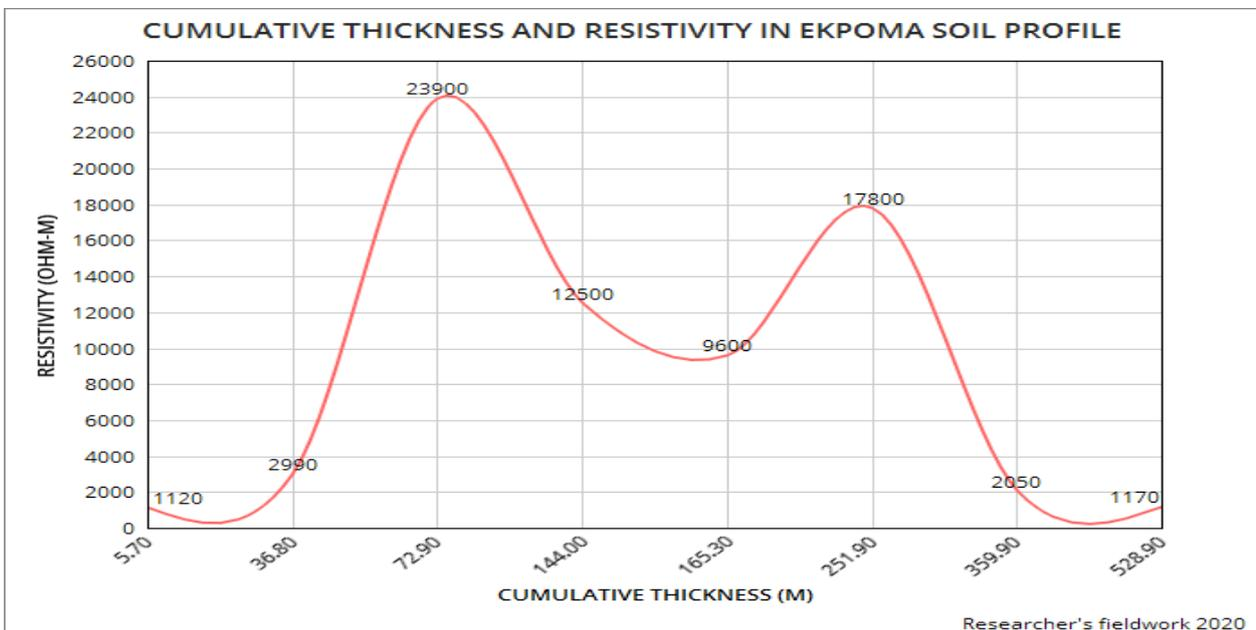
Fig. 3: Variations of apparent resistivity with cumulative thickness in Ekpoma Soil Profile (Culled from Table 1)
