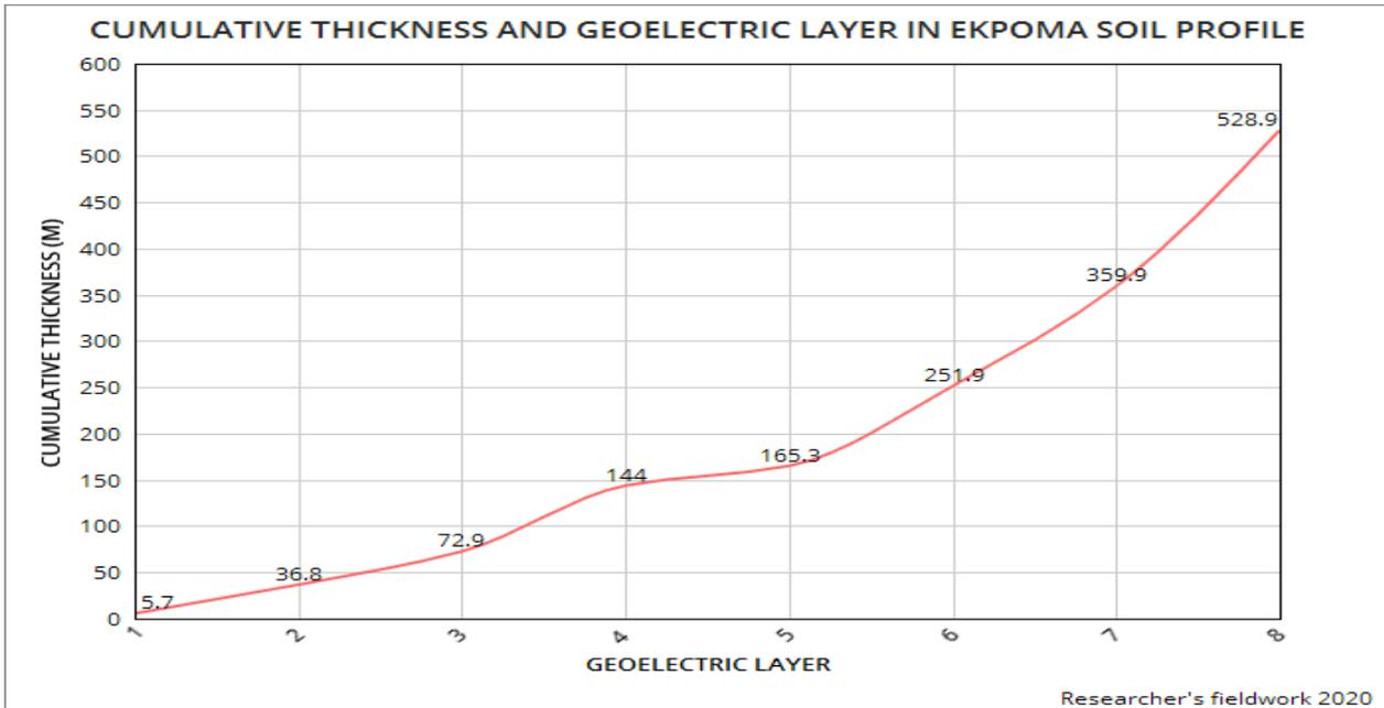
Fig. 2: Variations of cumulative thickness with geoelectric layer in Ekpoma Soil Profile (Culled from Table 1)
