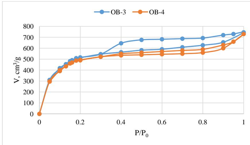
Rice. Fig. 1. Nitrogen adsorption isotherms on the studied samples.
